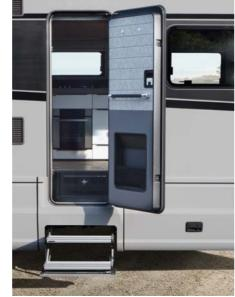
1 Smart body door with a sensor-controlled opening angle For trouble-free loading and unloading of the drawer units, we have equipped our body door with smart sensor technology. When the storage flap is open, the body door opens no further than 90°. This keeps the door and flap from colliding and is what makes such a large storage space next to the door even possible. It's unique technology that we have registered for a patent.
