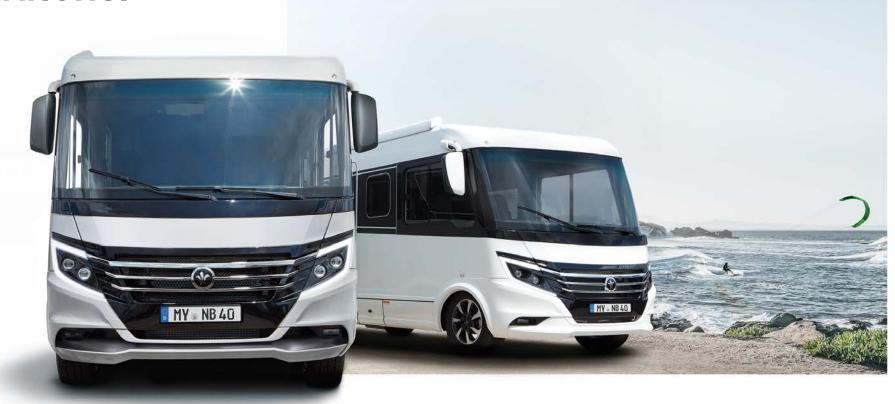
It is said that quality has its price, and it most particularly has its weight. High-quality materials in the iSmove such as two-sided aluminium sandwich walls with Styrofoam insulation plus a roof coating, rear panel and front mask made of GRP simply weigh a lot more than lower quality components. And while reducing weight was important, our top priority was to always uphold our customary Niesmann+Bischoff standards of quality. So how did we manage to do it? That will remain our little secret.
