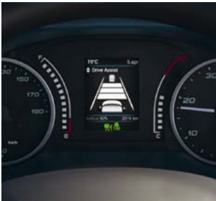
V2027811 Adaptive cruise control with emergency brake assistant
