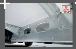
Dethleffs Lifetime-Plus: GRP-clad, wood-free underfloor, side walls with PU strips and XPS insulation
