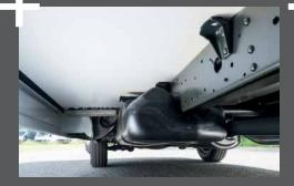
Durable, Lifetime-Plus bodywork construction without wood inserts! GRP-clad underfloor.
