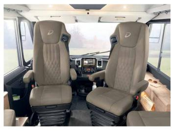
High-quality SKA captain seats are fitted as standard. As an option, hydraulic seats can be selected – to completely eliminate vibrations and bumps from the road surface. They can also be combined with seat heating and ventilation
