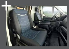
Ergonomic captain seats, multiadjustable, with seat heating and hydraulic suspension
