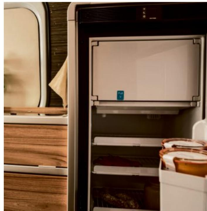
*The large compressor refrigerator in the Grand Canyon S with integrated freezer compartment has a capacity of 90 litres.*
