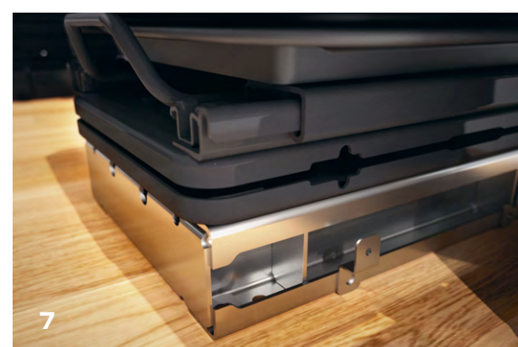
Seat consoles 42 per cent lighter – and yet even stiffer. By reinforcing our seat consoles and optimising their weight, we were able to reduce their structural deformation during a crash by 95 per cent. Two built-in arrestor hooks in each seat console provide additional support in the event of an impact.
