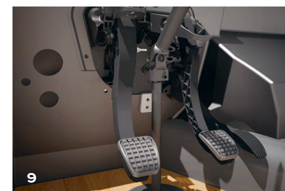
Pedal Release System Conventional pedals can injure the driver's legs in the event of a rear-end collision. Our pedal release system drastically reduces this risk – in the event of an impact, the pedals simply fold forwards out of the way.
