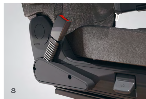
Seatbelt pretensioners To provide maximum safety, the seatbelts must restrain the occupants and tighten as early as possible. The integrated seatbelt pretensioners tighten the seatbelt in a fraction of a second to reduce the risk of injury.
