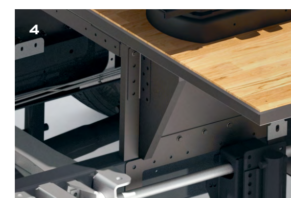
Platform In order to provide our liner with a completely insulated interior floor, the entire driver's cab has been raised onto a platform. The construction consists of aluminium sandwich panels as well as canted steel plates and is specifically designed to handle the loads generated during a crash.
