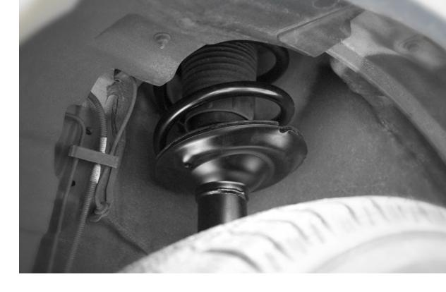
Reinforced coil springs are used in motorhomes with a heavy front axle load, whereas the RouteComfort comfort suspension strut finds use in light vehicles.
