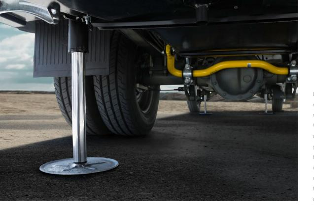
Depending on the vehicle type, we can offer you three varieties of struts: Tele-Star, Swing-Star and Vertical-Star. The central hydraulic unit is located in the interior of your motorhome, protecting it from harmful environmental influences. The emergency operation mode is a standard feature and allows for manual operation using a hand pump.
