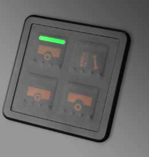
For ambulances and vehicles in commercial use, we offer an optional durable key-operated module. The module, which also works via the CAN bus, offers only those functions needed in rescue vehicles: Driving mode, offroad mode and service mode. To meet the requirements of vehicle manufacturers, the AirDriveControl® provides an additional switch input on the control unit. This lets you also control the air springs using a proprietary operating element of the manufacturer.
