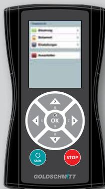
The Comfort control unit gives you an indication of the options waiting to be used in a CAN Bus-controlled system. Unlike the Basic version, the Comfort version has a large colour display. Simple menu navigation provides quick access to all of the available functions. In addition to the familiar "Automatic" and "Manual" modes, you can save and use individually set levels as needed. You can protect the system against unauthorised access using a PIN. This function also serves as an immobiliser.
