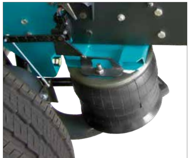
The full air spring system facilitates comfortable damping of the front and rear axle. The mighty air bags balance out unevenness in the road and iron out hard impacts gently, directing the spring forces through the sturdy steel construction to the vehicle frame.
