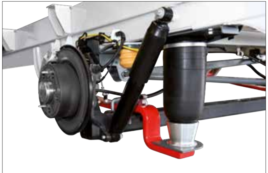
The full air spring system for the Fiat Ducato is available for the front and rear axle. The combination provides maximum driving comfort for your vehicle. The new air spring AirDriveControl® unit guarantees you comfortable and intuitive operation of your air spring system.
