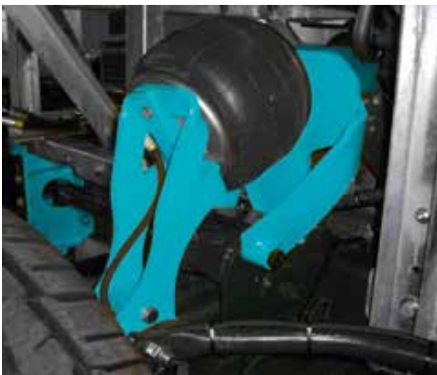
The full air spring system facilitates comfortable damping of the front and rear axle. The mighty air bags balance out unevenness in the road and iron out hard impacts gently, directing the spring forces through the sturdy steel construction to the vehicle frame.
